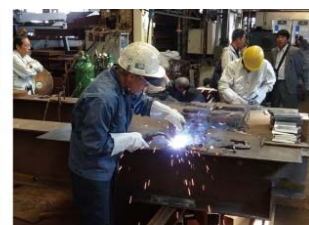
④仮組立て
